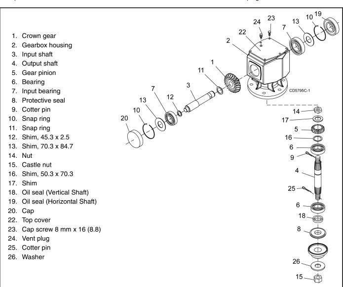
Figure 18. Gearbox Assembly
